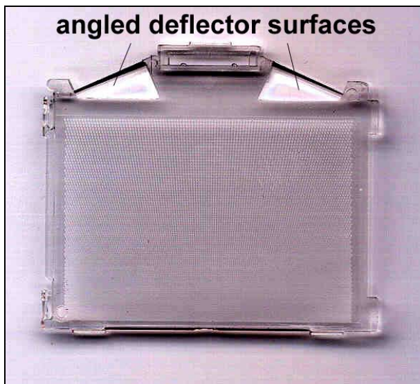
Figure 16: Lightguide with structure, 2 LEDs located under the angled deflector surfaces
