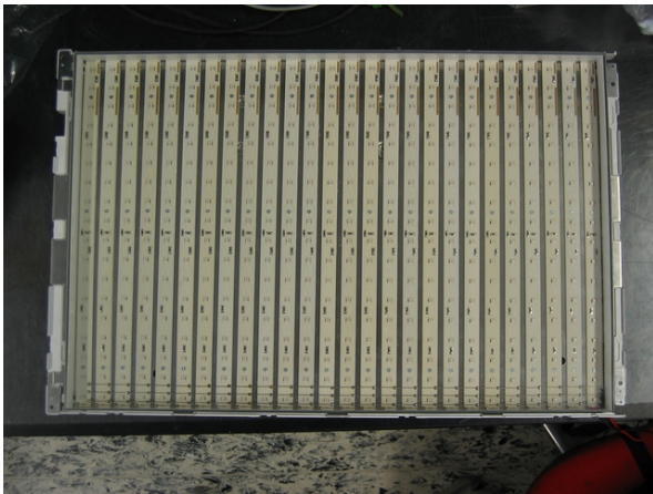
Figure 10a: Photo of the backlight (without optical films)
