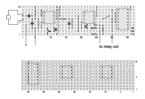
The sensitivity of the circuit can be adjusted using the variable potential divider connected to the inverting input of the comparator. To set the sensitivity to *maximum*, connect a voltmeter to the output of the second amplifier and adjust the variable potential divider to the point which *just* takes the voltmeter reading to its lowest figure (zero for CA3140, about 1.5v for TL081).
