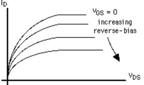
A still more extended range of variation of the drain characteristics is sketched to the right. The voltagecontrolled (VCR) region, i.e., operation before pinch-off, is conventionally called (mostly) just that, i.e., VCR region. The 'constant' current (pinch-off) region to the right is 'saturation' (probably all the remarks respecting a conflict with BJT terminology already have been said, repeatedly).
