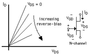
The conventional JFET icon for an N-channel device also is shown in the figure, and is identified as to type by the gate terminal PN junction arrow. Note that following common convention the drain current is positive (in the direction of the current polarity arrow shown) for an electron carrier flow from source to drain.
