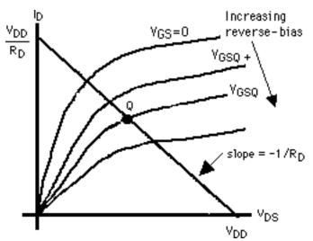
Suppose now the gate voltage is changed, say increased (i.e., made less negative) to  $V_{GS+}$ . There is a consequent increase in drain current, an increase in the voltage drop across the drain resistor, and a <u>decrease</u> in the drain-source voltage. Locating the new operating point graphically is a matter of moving 'up' the load line to the transistor characteristic identified by the gate voltage  $V_{GS+}$ .
