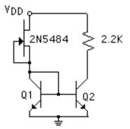
6) The current source of problem 4 is relatively constant for voltages above the pinchoff voltage (and below gate-drain breakdown). However channel length modulation introduces a slope to the drain characteristic, corresponding to a finite equivalent source resistance. The circuit shown to the left uses feedback to effectively increase this resistance. The drain characteristics on the right are used to illustrate the feedback action.
