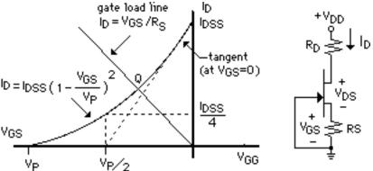
for an incremental signal, the short-circuit connection really is inappropriate. However the gate leakage current is quite small (about 1 nanoampere for the 2N5484) so that a rather large resistor can replace the short-circuit connection to provide an input resistance across which there is a negligible voltage drop due to the gate current.
