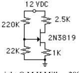
8) The JFET in the circuit shown has manufacturing tolerances such 15ma, and -5v Vp -2v. Bias the device so that that 10ma IDSS 8ma ID 6ma; neglect channel-length modulation. Compute bias currents and voltages for your calculated element values using the 2N3819 JFET (IDSS=11.6ma, Vp=-3v).
