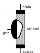
By convention the terminal designations are defined so that carriers (electrons for the N-channel device) flow <u>from</u> the source and <u>to</u> the drain. For the N-channel device, therefore, a voltage is assumed to be applied so that the drain is positive relative to the source.
