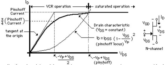
The tangent line from the origin and the saturation current provide convenient asymptotes with which to sketch a characteristic fairly accurately; note again that the actual current is 3/4 that at the intersection of the asymptotes.
