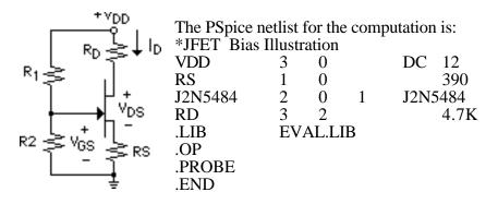
The biasing analysis may be computed by calculating the drain current (saturation) as a function of the gate-source voltage; the plot below is for  $V_{DS} = 12$  volts. Note that IDSS differs somewhat from the nominal value of 2.41 ma because of the channel length modulation.
