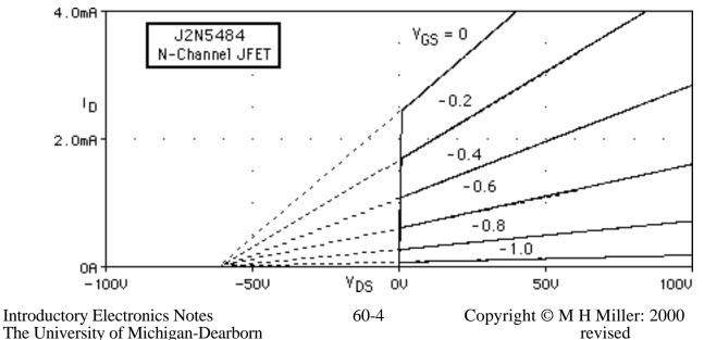
The 'channel-length modulation effect causes the characteristics to converge at a common intersection, about -60 volts for the 2N5484.
