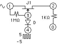
Conversely if the node 1 voltage is negative node 2 acts as the drain. The gate is reverse biased but only slightly so because the leakage current is small. Again the low channel resistance means the node 2 voltage tracks the node 1 voltage.
