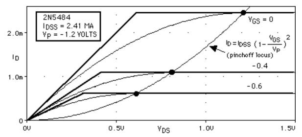
To obtain an <u>estimate</u> of the channel resistance in the VCR region (for small values of V<sub>DS</sub>) we can use the ratio of coordinates of the asymptote intercept point, i.e., the slope of the tangent at the origin.. For the VGS = 0 characteristic this estimate is  $(-V_P/2)/I_{DSS} = (1.21/2)/.00241 = 251$ ; the resistance increases for more negative gate voltages.
