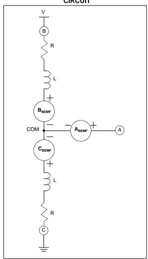
Figure 7 shows the equivalent circuit of the motor with coils B and C driven while coil A is undriven and available for BEMF measurement. At the commutation frequency the L's are negligible. The R's are assumed to be equal. The L and R components are not shown in the A branch since no significant current flows in this part of the circuit so those components can be ignored.
