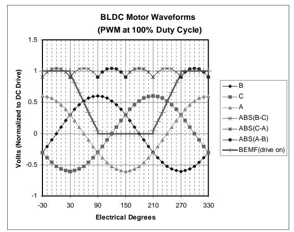
Notice that the BEMF(drive on) waveform is fairly linear and passes through a voltage that is exactly half of the applied voltage at precisely 60 degrees which coincides with the zero crossing of the coil A BEMF waveform. This implies that we can determine the rotor electrical position by detecting when the open terminal voltage equals half the applied voltage.
