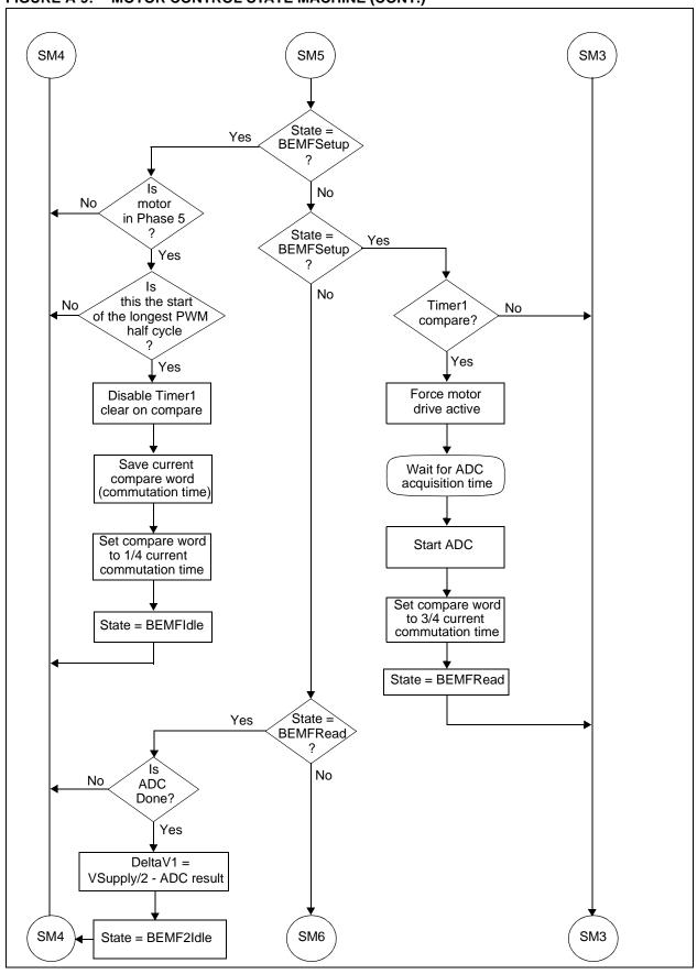
FIGURE A-9: MOTOR CONTROL STATE MACHINE (CONT.)
