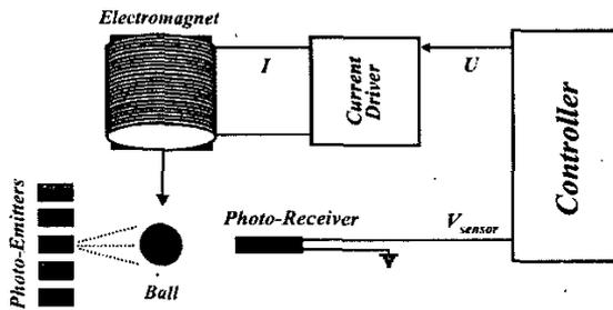
Fig. 2. Main components of the magnetic levitation system
