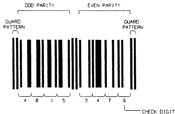
Figure 0-9 : EAN 8 Symbol Encoding the Data "4015347."
