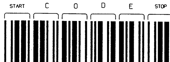
Figure 0-13 : Code 39 Symbol Encoding The Data "CODE"
