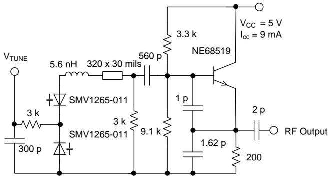
Figure 7. VCO Circuit Diagram
