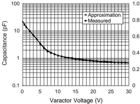
Figure 5. SMV1265 Capacitance vs. Voltage
