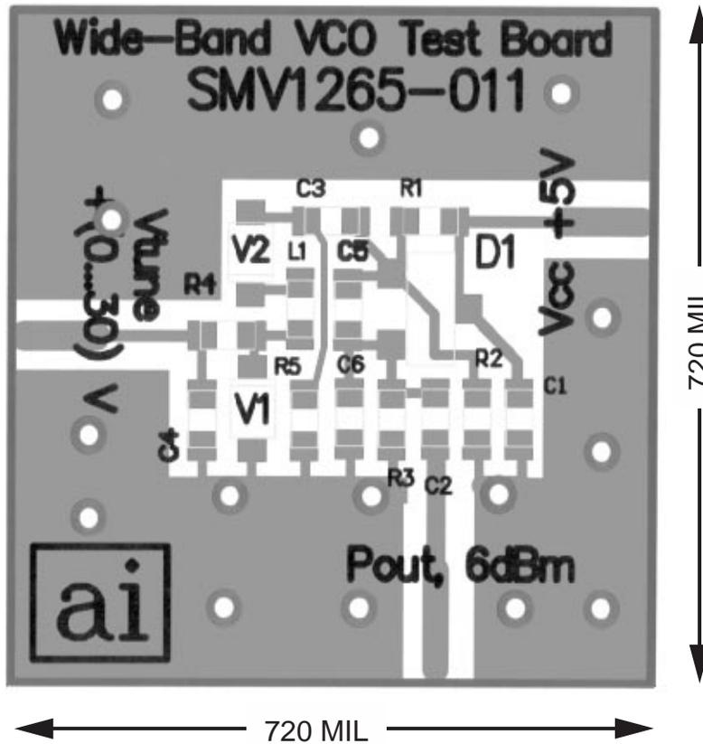
Figure 8. PCB Layout
