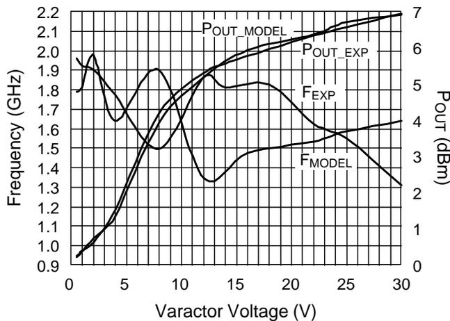
**Figure 9. Measured and Simulated Frequency vs. Varactor Voltage**
