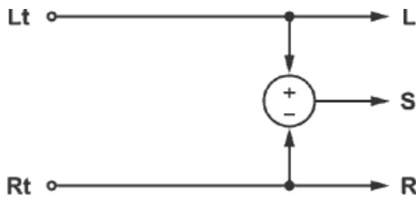
**Figure 2** Simple passive surround decoder concept
