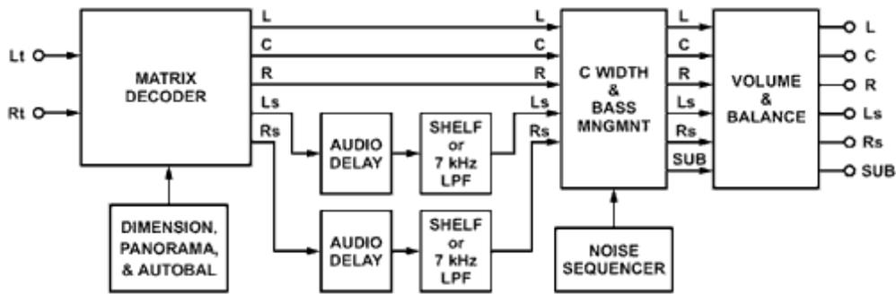
**Figure 5** Basic decoder system block diagram
