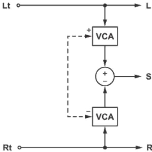
**Figure 3** Decoder with VCA balancing
