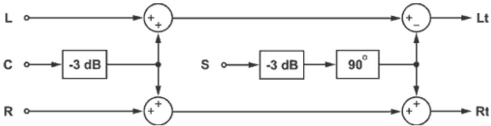
**Figure 1** Simple four-input encoder concept
