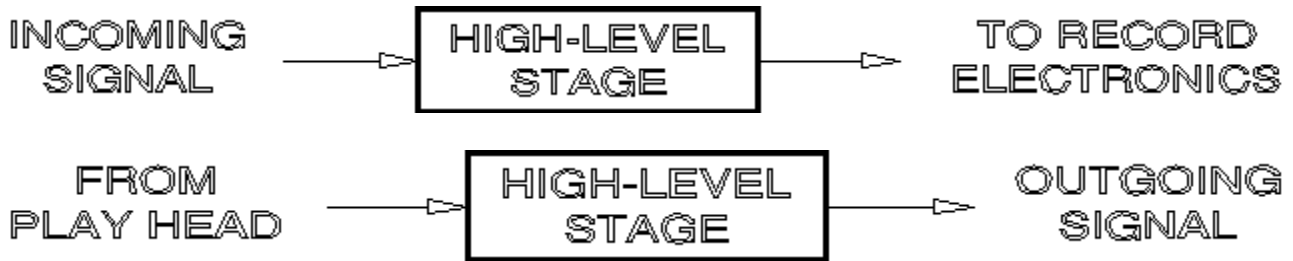
Figure 5. B-type noise reduction system-block diagram.
