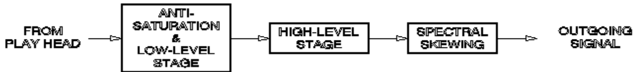
Figure 9. The Dolby C-type noise reduction block diagram.
