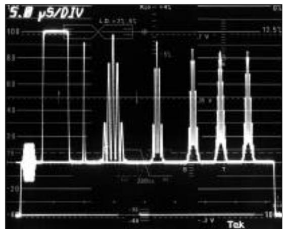
Figure 48. The multipulse signal exhibiting high frequency roll-off.
