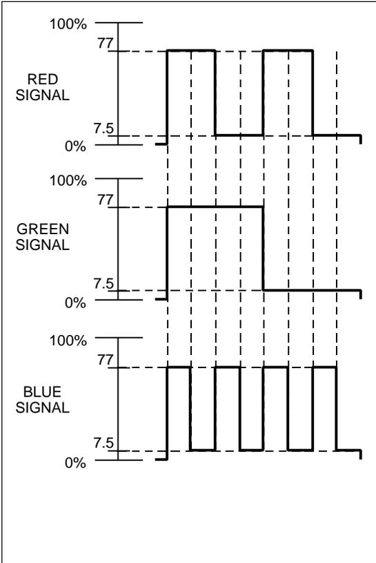
Figure 110. RGB levels decoded from 75% bars with 75% white.
