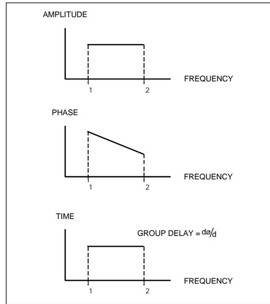
Figure 57. Response of a distortion free system.
