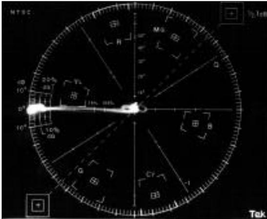
Figure 74. A vectorscope display indicating 15% differential gain.
