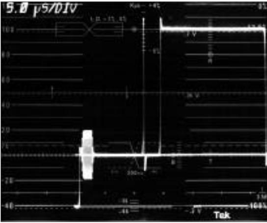
Figure 63. The 1780R graticule indicates 2%  $K_{pulse/bar}$ .
