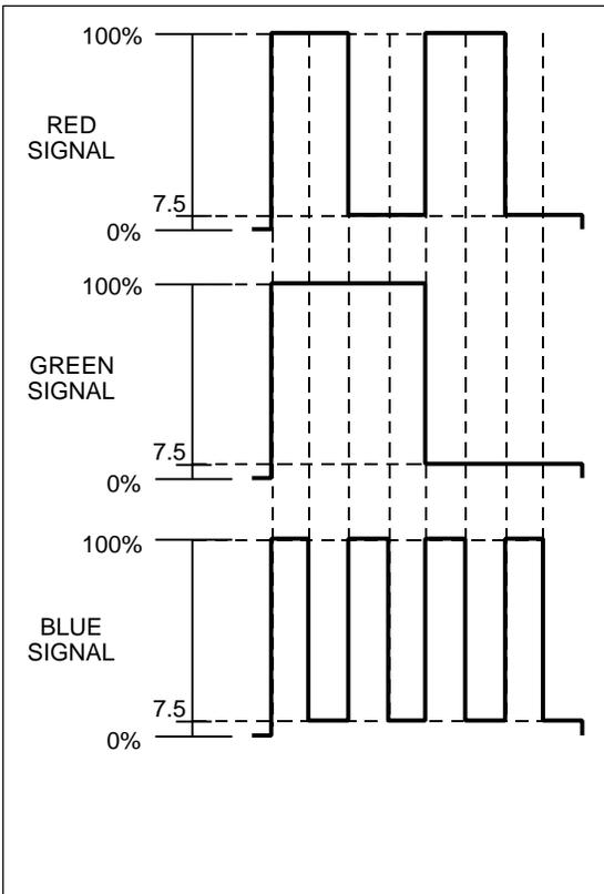
Figure 111. RGB levels decoded from 100% bars with 100% white.
