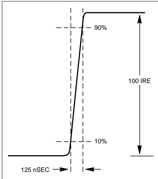
Figure 26. A T rise time bar has a 10% to 90% rise time of 125 nanoseconds.
