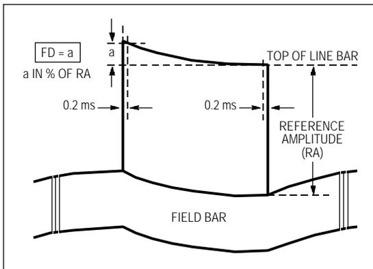
Figure 36. Parameters for measurement of field time distortion.
