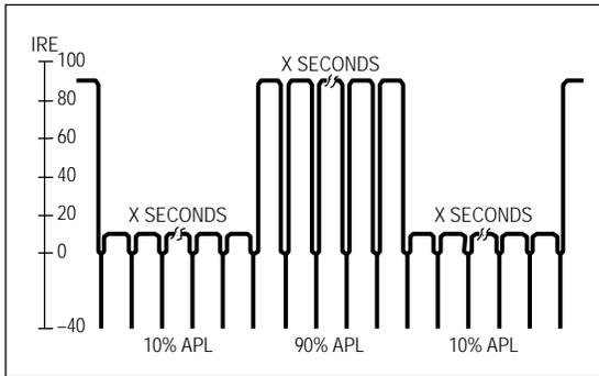
Figure 94. A flat field bounce test signal.
