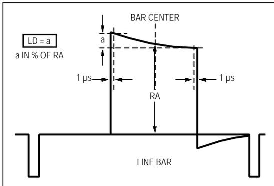
Figure 32. Parameters for measurement of line time distortion.
