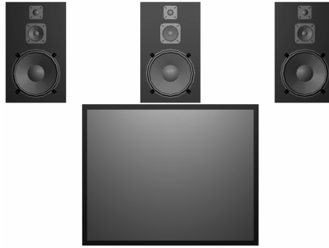
Figure 2-12 Ideal Setup—All Speakers Above Screen
