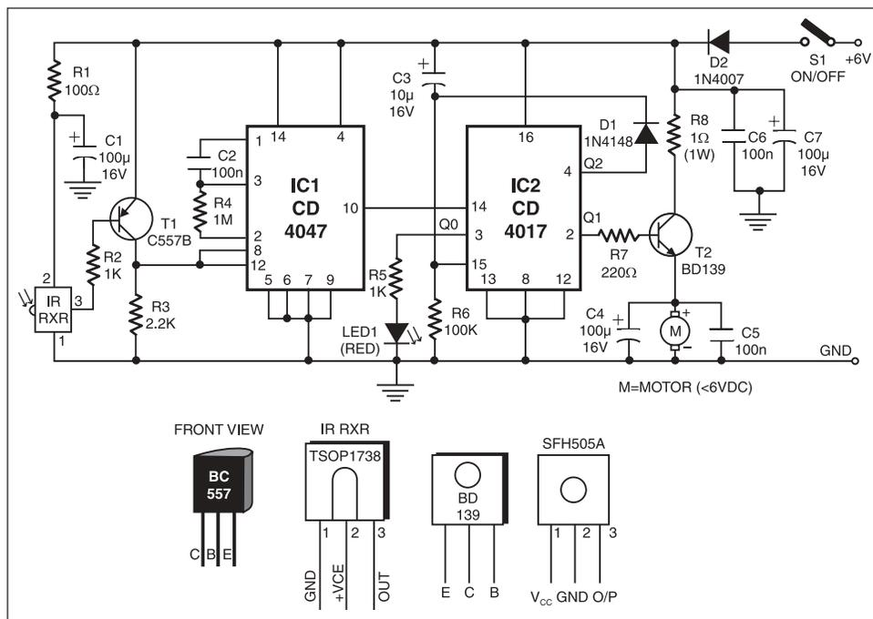
This circuit can be easily fabricated on a general-purpose printed board. After construction, enclose it inside the toy car and connect the supply wires to the battery of the toy car with right polarity. Rewire the DC motor connections and fix the IR receiver module in a suitable location, for
