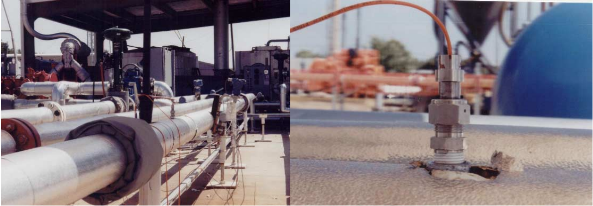
Figure 12.9. Fiber optic flow sensor deployment in outdoor flow loops of Tulsa University, OK.
