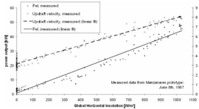
Fig. 8 Manzanares solar tower prototype input/output characteristics
