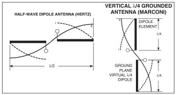
Figure 5: Dipole Antenna Operation
