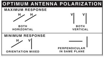
Figure 11: Antenna Polarization
