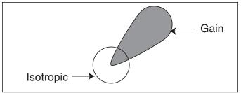
Figure 10: Antenna Gain
