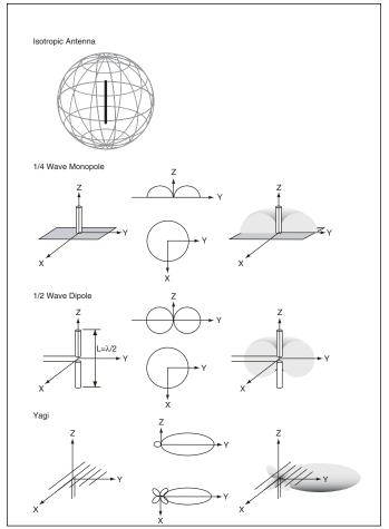
Figure 8: Antenna Radiation Patterns
