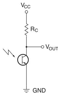
**Figure 1. Common-Emitter Amplifier**
