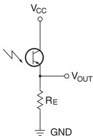
**Figure 2. Common-Collector Amplifier**
