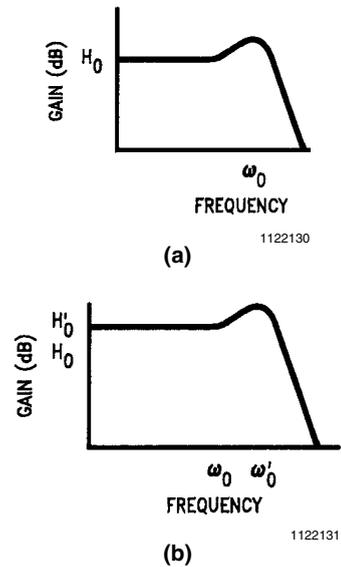
**FIGURE 20. Effect of changing  $H_0$  and  $\omega_0$ . Note that, when log frequency and gain scales are used, a change in gain or center frequency has no effect on the shape of the response curve. Curve shape is determined by Q.**
