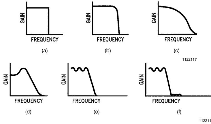
FIGURE 11. Examples of Low-Pass Filter Amplitude Response Curves
