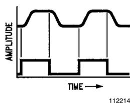
**FIGURE 28.** Response of a 4th-order Bessel low-pass (upper curve) to a square wave input (lower curve). Note the lack of ringing in the response. Except for the "rounding of the corners" due to the reduction of high frequency components, the response is a relatively undistorted version of the input square wave.
