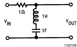
FIGURE 6. Example of a Simple Notch Filter
