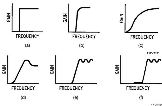
FIGURE 14. Examples of High-Pass Filter Amplitude Response Curves
