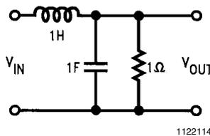
FIGURE 9. Example of a Simple Low-Pass Filter
