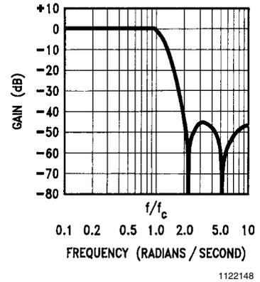
FIGURE 31. Example of an elliptic low-pass amplitude response. This particular filter is 4th-order with  $A_{max} = 0.5$  dB and  $f_s/f_c = 2$ . The passband ripple is similar in form to the Chebyshev ripple shown in *Figure 25(c)*.
