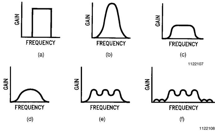
FIGURE 5. Examples of Bandpass Filter Amplitude Response
