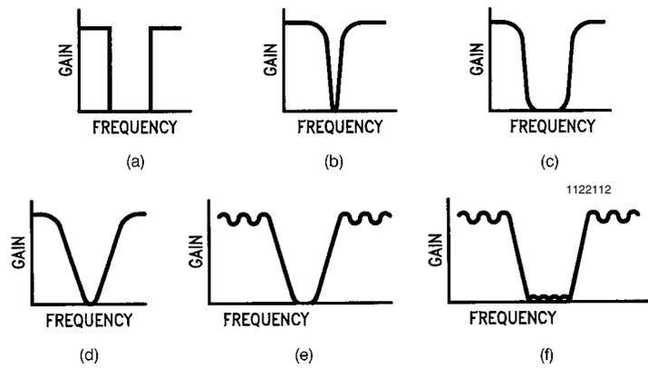
FIGURE 8. Examples of Notch Filter Amplitude Responses
