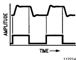
**FIGURE 27.** Response of a 4th-order Butterworth low-pass (upper curve) to a square wave input (lower curve). The "ringing" in the response shows that the nonlinear phase shift distorts the filtered wave shape.
