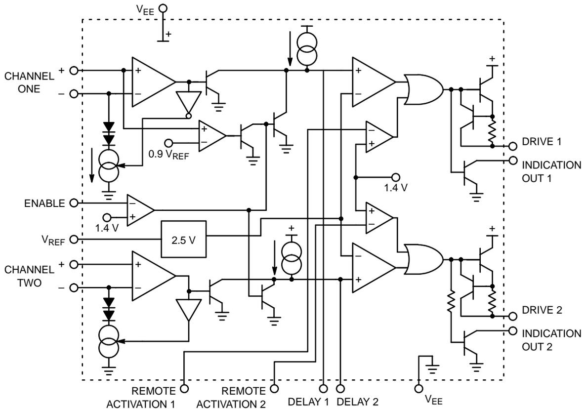
Figure 17. MC3424/MC3524 Equivalent Circuit
