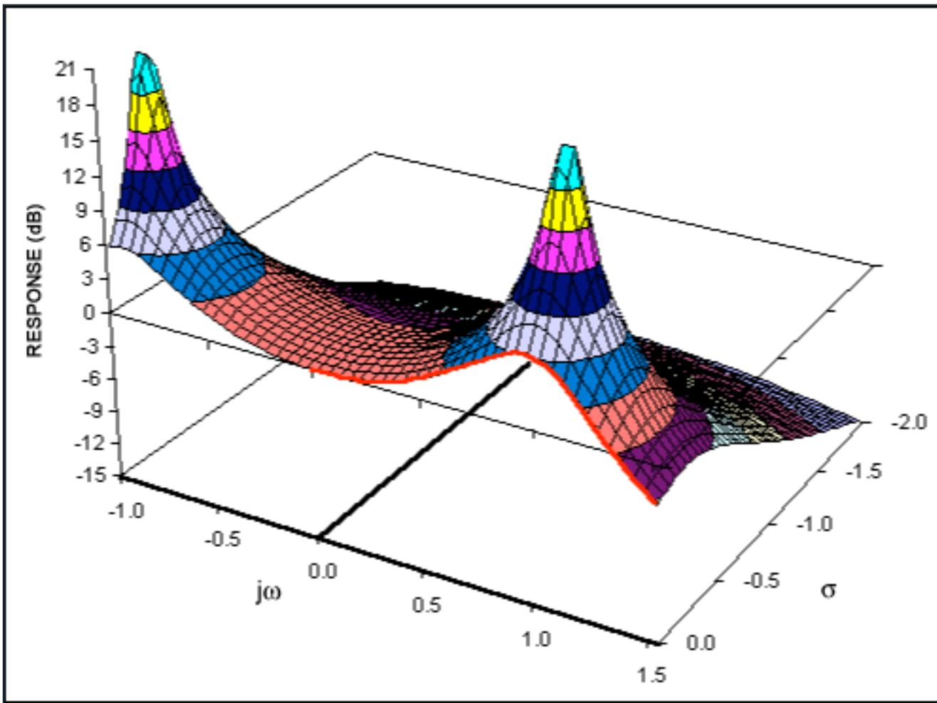
Figure 4b. The complex function of a second-order lowpass filter ( $Q = 2$ ).
