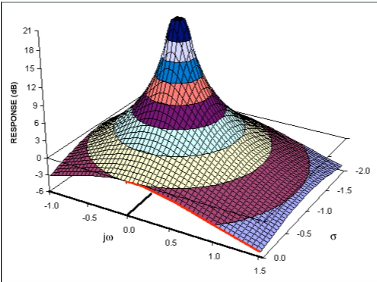
Figure 2b. The complex function of an RC lowpass filter.
