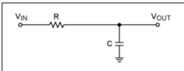
Figure 2a. A simple RC lowpass filter.
