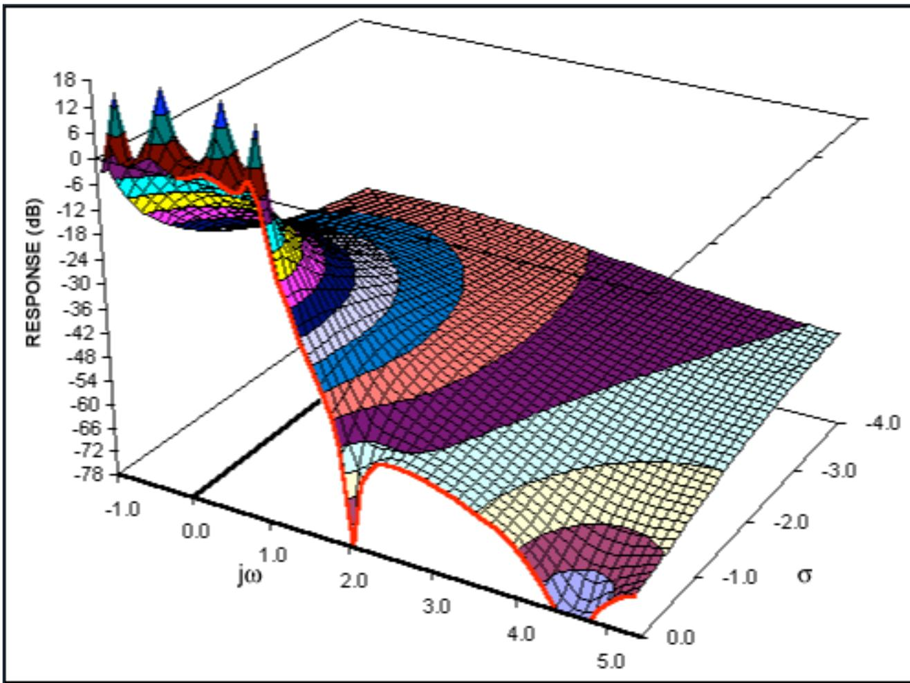
Figure 10b. The complex function of a fourth-order elliptic lowpass filter.
