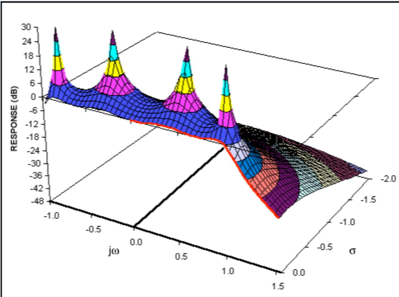
Figure 8b. The complex function of a fourth-order Chebyshev lowpass filter.
