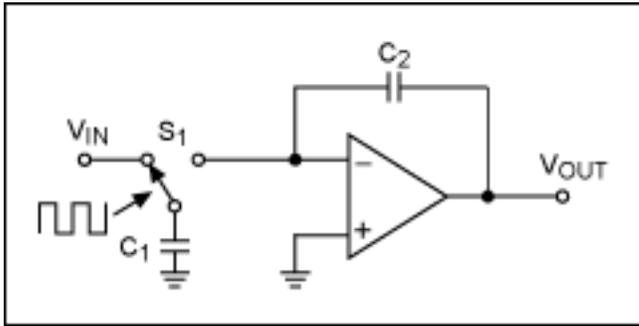
Figure 12. A switched-capacitor integrator.
