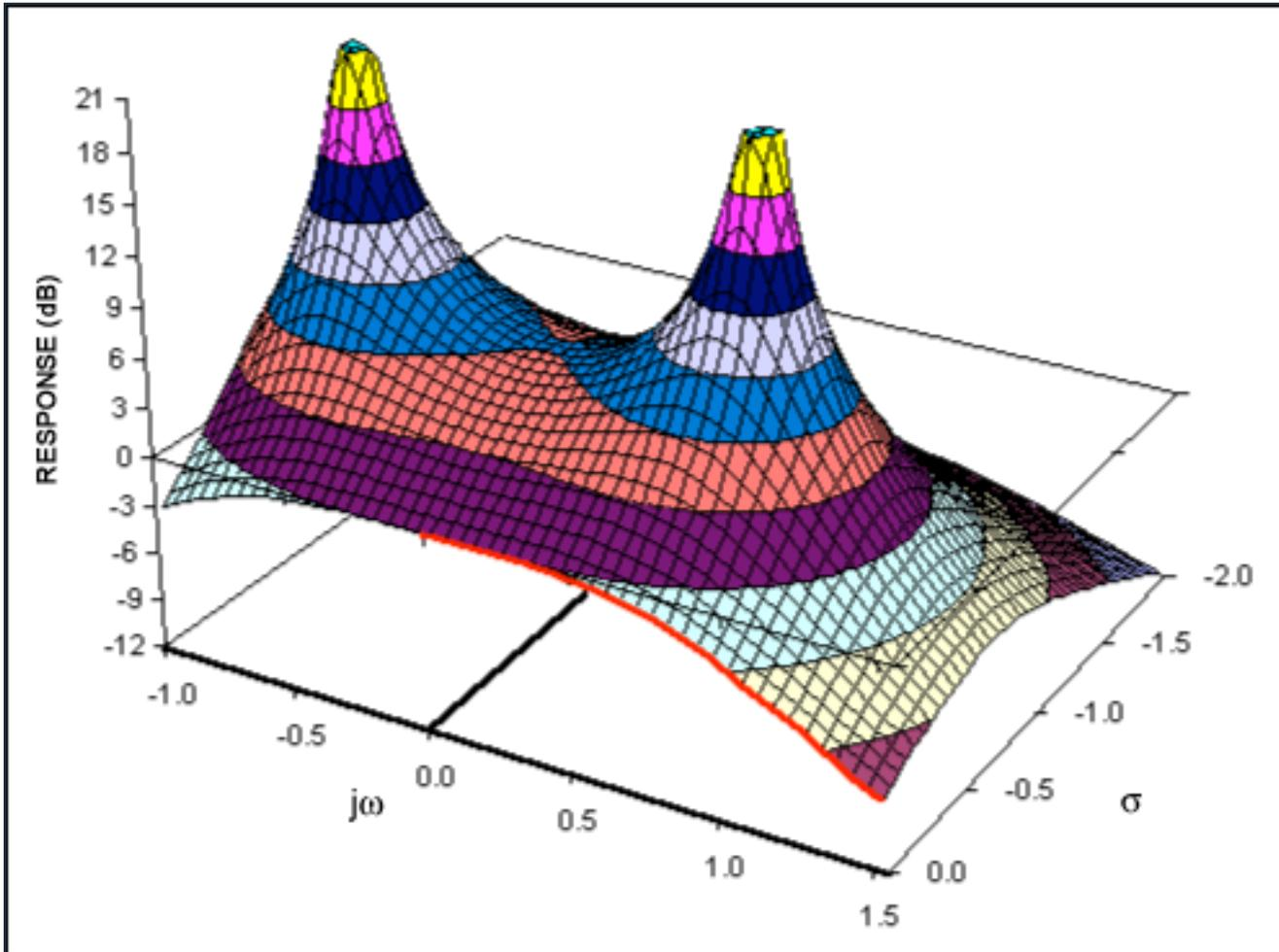
Figure 4a. The complex function of a second-order lowpass filter ( $Q = 0.707$ ).
