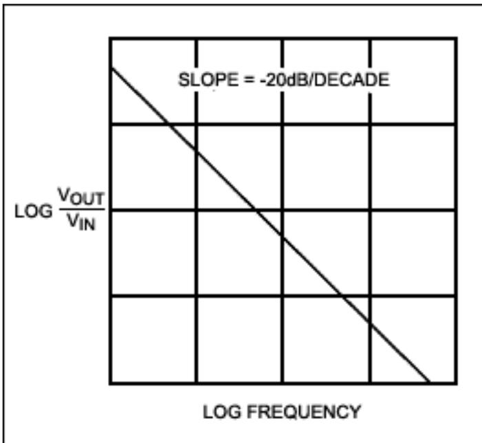
Figure 1b. A Bode plot of a simple integrator.
