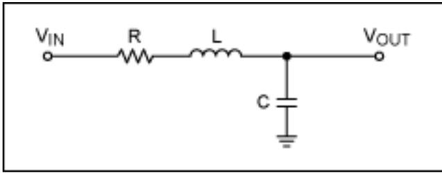
Figure 3a. An RLC lowpass filter.
