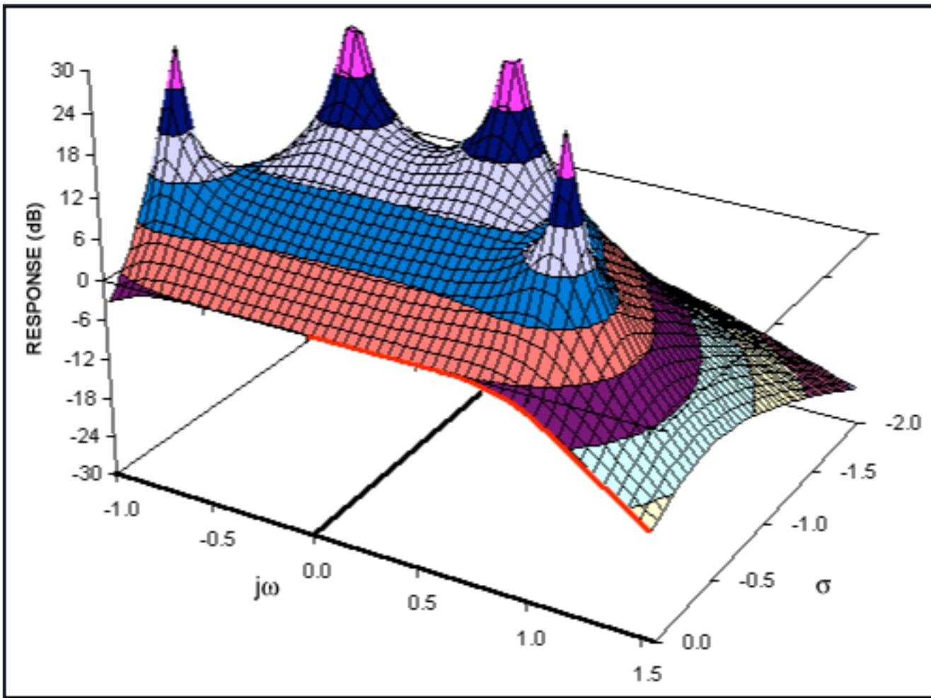
Figure 7b. The complex function of a fourth-order Butterworth lowpass filter.
