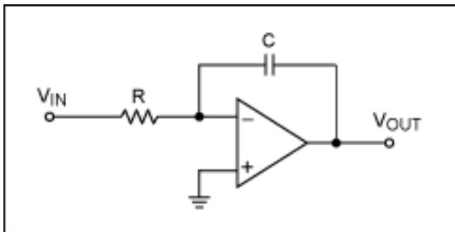
Figure 1a. A simple RC integrator.
