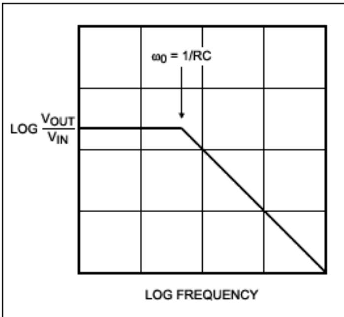
Figure 2c. A Bode plot of a lowpass filter.
