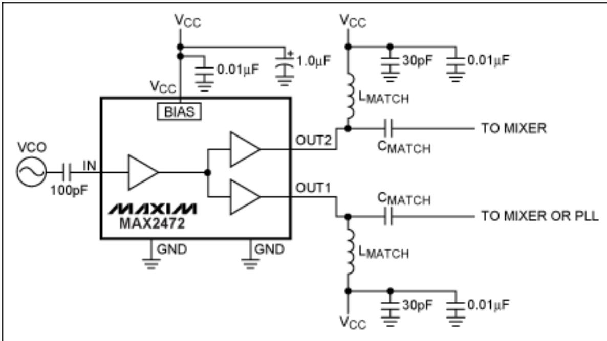
Figure 13. MAX2472 typical operating circuit.
