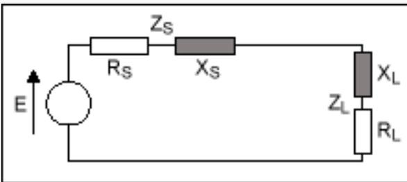
Figure 2. Diagram of  $R_S + jX_S = R_L - jX_L$ .
