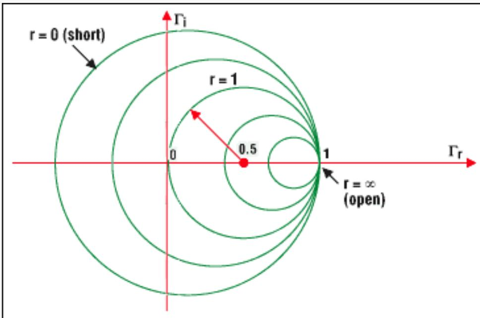
Figure 4a. The points situated on a circle are all the impedances characterized by a same real impedance part value. For example, the circle,  $r = 1$ , is centered at the coordinates  $(0.5, 0)$  and has a radius of  $0.5$ . It includes the point  $(0, 0)$ , which is the reflection zero point (the load is matched with the characteristic impedance). A
