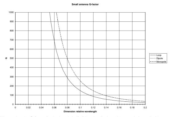
We see that the Q-factor for the loop is half of that the dipole and monopole have. In this respect the loop utilises the physical dimensions more efficiently than the dipole and monopole. This can be explained by the two-dimensional structure of the loop, while the monopole and dipole are one-dimensional structures only (a string).
