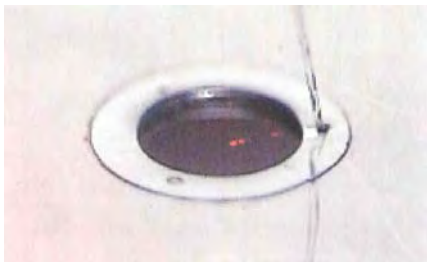
Fig.12-7 Bottom element of liquid immersion objective.
