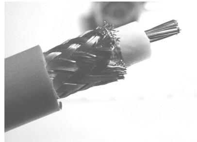
4) Slide outer ring onto cable as shown. Do not comb out braid.
