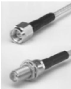
*SMA* is an acronym for SubMiniature version A and was developed in the 60s. 50  $\Omega$  SMA connectors are precision, subminiature units that provide excellent electrical performance up to 18 GHz. These high-performance connectors are compact in size and mechanically have outstanding durability.
