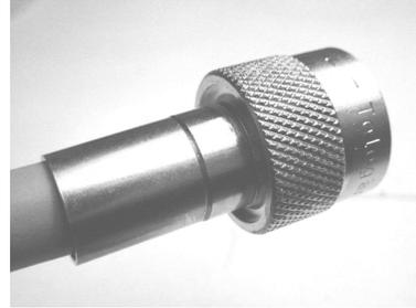
8) Crimp outer ring using the crimping tool. It is a one-shot operation, so be careful in positioning the tool properly around the ring and press strongly. If necessary, you can crimp the ring few more times.
