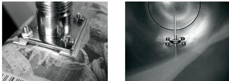
10) You can use this antenna as a feeder for a Parabolic Dish. To match the feeder with the optimal dish size, keep in mind that the horizontal and vertical 3dB beamwidths are given by:
