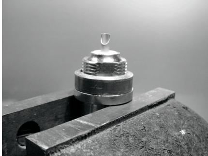
8) Screw the nut to the connector to fix it firmly on the plate using the spanner.
