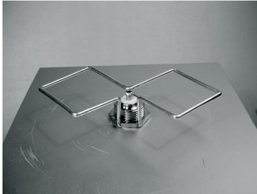
17) We now want to solder the central pin of the connector to the center of the shaped wire. You may have either a short or long type of N connector, as shown.
