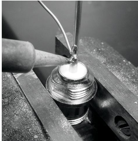
6) Insert a washer and screw gently the nut on the connector. Trim the wire at 3.05 cm measured from the bottom part of the nut.
