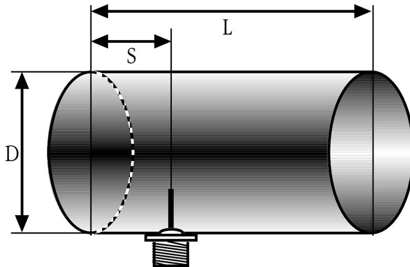
a) The acceptable values for the diameter  $D$  of the feed are between 0.60 and 0.75 wavelength in air at the design frequency. At 2.44 GHz the wavelength  $\lambda$  is 12.2 cm, so the can diameter should be in the range of 7.3 - 9.2 cm.
