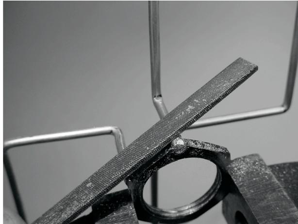
16) Insert the connector into the hole of the metallic plate and screw the nut with the wire soldered on it.
