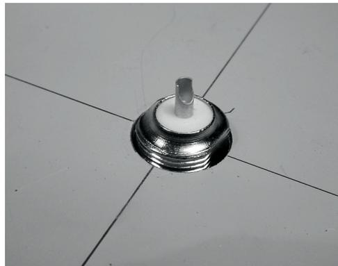
7) To have an antenna impedance of 50 Ohms, it is important that the visible surface of the internal insulator of the connector (the white area around the central pin) is at the same level as the surface of the plate. For this reason, cut 0.5 cm of copper pipe with an external diameter of 2 cm, and place it between the connector and the plate.
