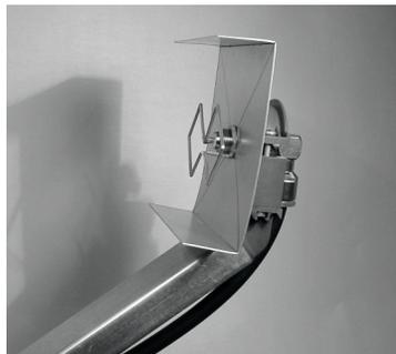
Other types of home-made directive antennas may be used as feeders for Parabolic Dishes. The important point is to match the beamwidth of the feeder with the dish size, and to place the feeder exactly in the focus of the dish.
