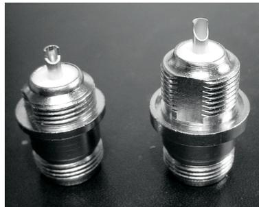
The central pin of the long type may be soldered directly on the shaped wire, while the short type of connector needs an additional short piece of straight wire to be soldered into the central pin.
