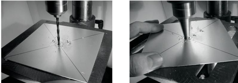
The hole should fit exactly the N connector. Use the file if needed.
