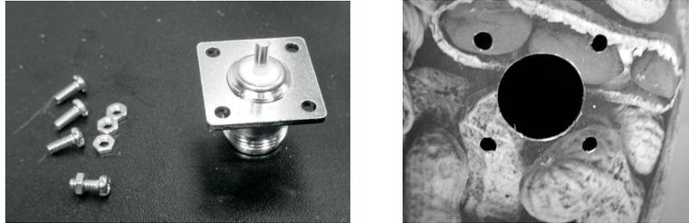
You should also use some additional washers (or thin metallic plates) in order to fit the flange on the curved surface of the can without changing its shape.
