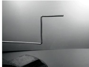
4) We will now twist the 'Z' portion of the wire to make a coil with a diameter of 1 cm. To do this, we will use the pipe or the drill bit and curve the wire around it, with the help of the vice and of the pliers.
