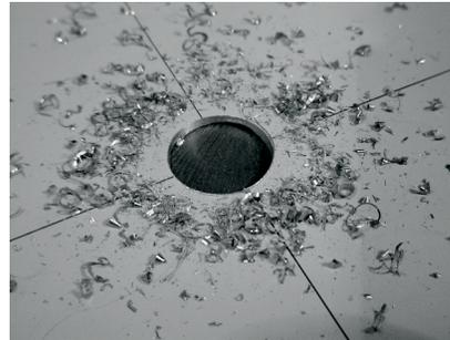
The hole should fit exactly the N connector. Use the file if needed.
