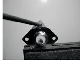
3) Power on the high power soldering iron and let it heat for a couple of minutes. Apply the soldering iron to the connector until it gets hot (really hot! Be very careful!), but avoid melting the dielectric. Then tin the area around and inside the holes by applying solder until it flows. Avoid filling the holes with solder. Tinning is required to facilitate the process of soldering the wires to the connector.
