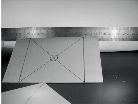
The lines between the central square and the two side rectangles should not be carved deeply on both sides with the cutter, but only on the upper side and just enough to facilitate the bending of the plate. The two lips should be folded at 90 degrees. Use the vice if needed.
