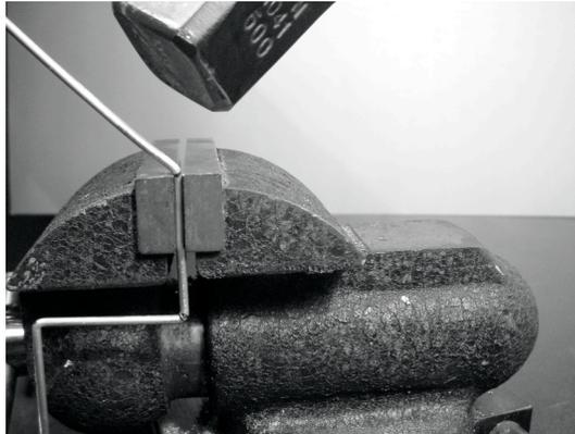
8) Draw now a line at 3.05 cm from the last edge, and a second line after 2.3 cm from the first one. Bend the wire at 90 degrees in the second line, in a direction orthogonal to the plane containing the wire, as shown.
