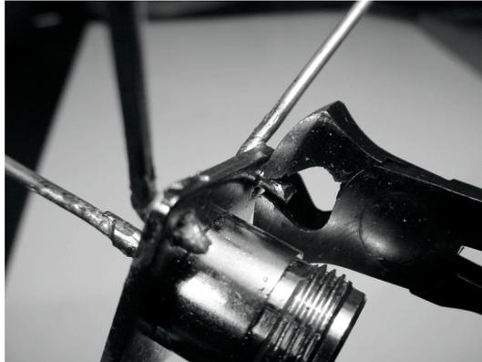
9) With the pliers, bent over the four radials at 30 degrees from the horizontal plane. This is done to match the impedance to 50 Ohms. To facilitate this operation, you may draw the 30 degrees angle on paper, and compare the antenna with it as shown.
