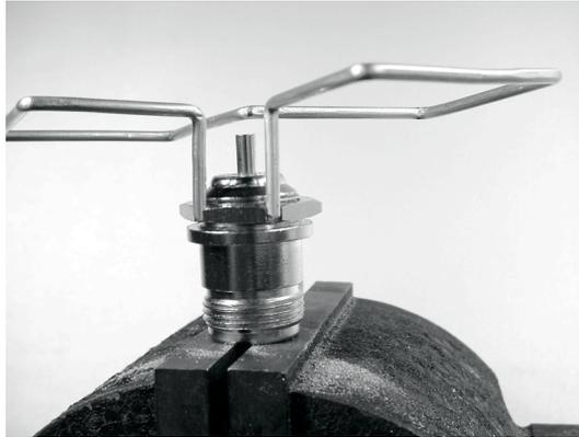
14) Tin the ends of the wire for 0.5 cm. Tin around and inside the cuts of the nut with a small amount of solder, and then solder the wires to the nut.
