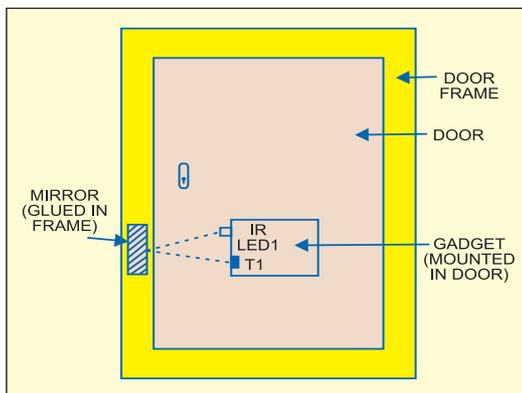
Fig. 3: Back view of the door assembly
