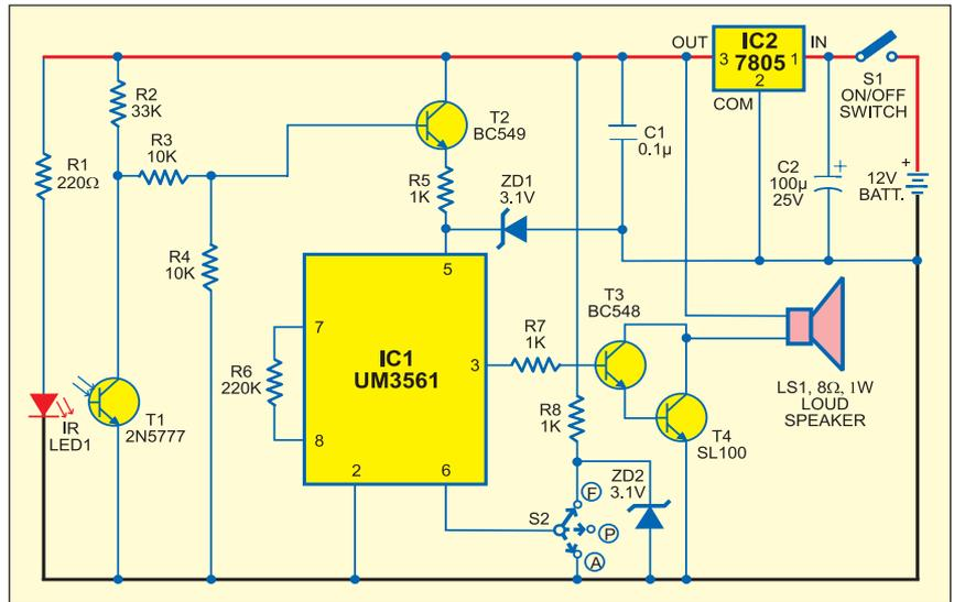
Fig. 1: Circuit of the door guard
