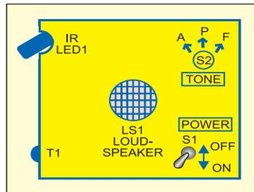
Fig. 4: Suggested enclosure with major components layout
