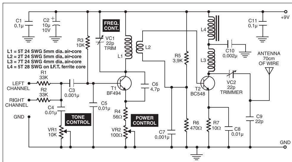
are to be wound over the same air core such that windings for coil L2 start from the end point for coil L1. Coil winding details are given below:
