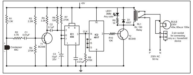
Here is a clap switch which is used to turn ON/OFF any appliance connected to it. The circuit changes its output state when you clap near the condensor mic.
