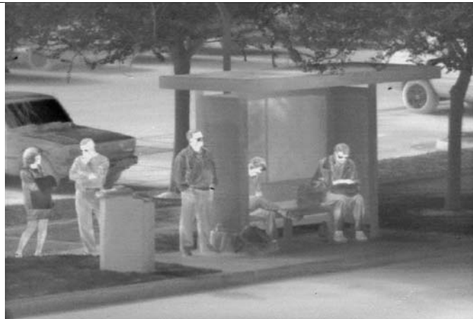
Fig. 10.10 An image taken by the camera developed by Raytheon based on their 640 \times 480 pixel \text{VO}_2 FPA, showing excellent resolution and image quality. After [80]
