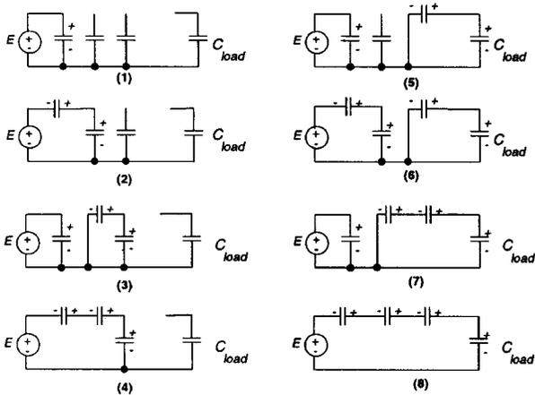
Fig. 5. A three-stage charge pump based on MPVDs .
