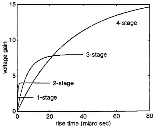
Fig. 15. Rise time optimization of TPVD charge pump.
