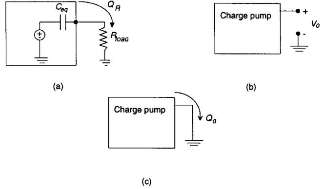
Fig. 9. The evaluation of the equivalent capacitance network.
