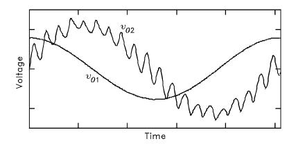
Figure 3: Output voltage waveforms for two different LC filter cutoff frequencies.
