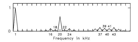
Figure 10: Spectrum of the output voltage  $v'_{\Omega}$ .
