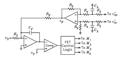
Figure 7: Input stage to the bridged amplifier with feedback.
