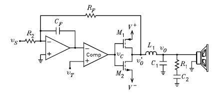
Figure 5: Amplifier with negative feedback.
