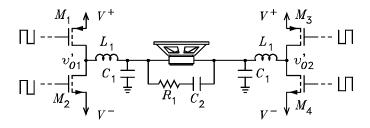
Figure 6: Bridged output stage.
