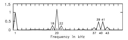
Figure 4: Unfiltered spectrum of the output voltage.
