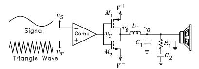
Figure 1: Basic class-D amplifier.
