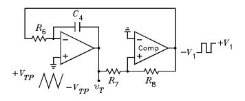
Figure 8: Triangle wave generator.
