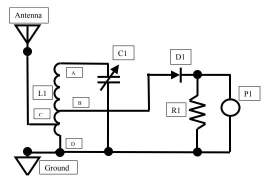
Antenna wire is 15' long medium sized clip on the end Ground wire is 10' long with large clip on end
