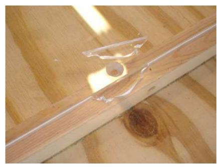
Oops! This photo shows a closeup of where the two halves of the plexiglass cover meet over the center divider. I drilled and countersunk holes all around the edges of both pieces of plexiglass so I could screw them onto the face of the panel
