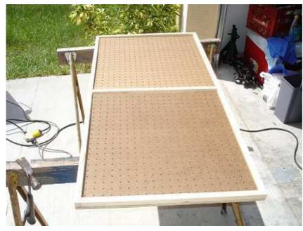
Next I cut two pieces of masonite pegboard to fit inside the wells. These pieces of pegboard will be the substrates that each sub-panel will be built on. They were cut to be a loose fit in the wells. You don't have to use peg-board for this. I just
