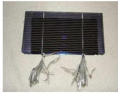
I bought a couple of bricks of 3 X 6 mono-crystalline solar cells. It takes a total of 36 of these type solar cells wired in series to make a panel. Each cell produces about 1/2 Volt. 36 in series would give about 18 volts which would be good for charging 12
