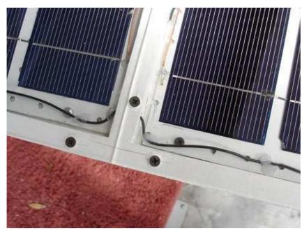
Wires to connect the two half panels together were run through the vent holes in the central divider. Again, blobs of silicone caulk were used to anchor the wire in place and prevent it from flopping around.
