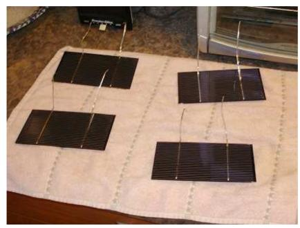
Here are some separated and cleaned solar cells drying on a towel. Once separated from their wax stabilized brick form, they are amazingly fragile and difficult to handle and store. I would recommend leaving them as bricks until you
