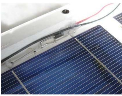
Each solar panel in a solar power system needs a blocking diode in series with it to prevent the panel from discharging your batteries at night or during cloudy weather. I used a Schottky diode with a 3.3 Amp current rating. Schottky diodes have a much
