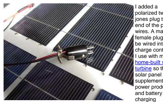
I added a polarized two-pin jones plug to the end of the panel wires. A mating female plug will be wired into the charge controller I use with my home-built wind turbine so the solar panel can supplement it's power production
