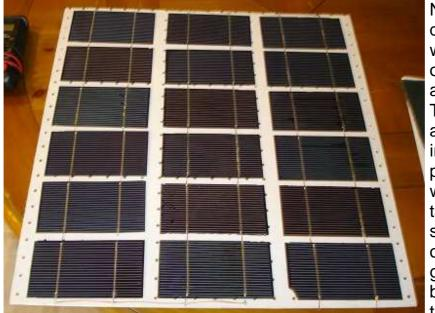
Next time I will do it differently. I will solder tabs onto the backs of all the solar cells. Then I will glue all the cells down in their proper places. Then I will solder the tabs together. It seems like the obvious way to go to me now, but I had to do it the hard way
