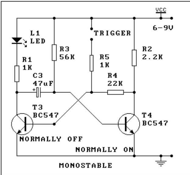
capacitor in the circuit which determines that T3 will be off, and T4 will be on in its stable state.
