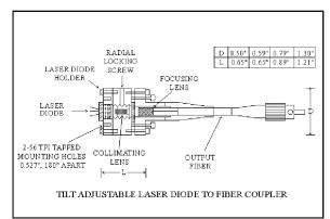
or vibration. In fact, tilt adjustable source couplers can be used over a temperature range of -25°C to 60°C, and have been vibration tested. Higher temperature versions are available on request.
