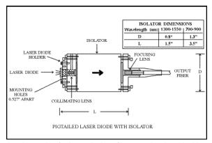
Another option for laser diode to fiber couplers is a blocking screw to attenuate the output beam. This allows the user to precisely control the output power entering the fiber, without having to change the diode current. Another option is laser diode to fiber couplers with polarizer or polarization Rotator in the middle.
