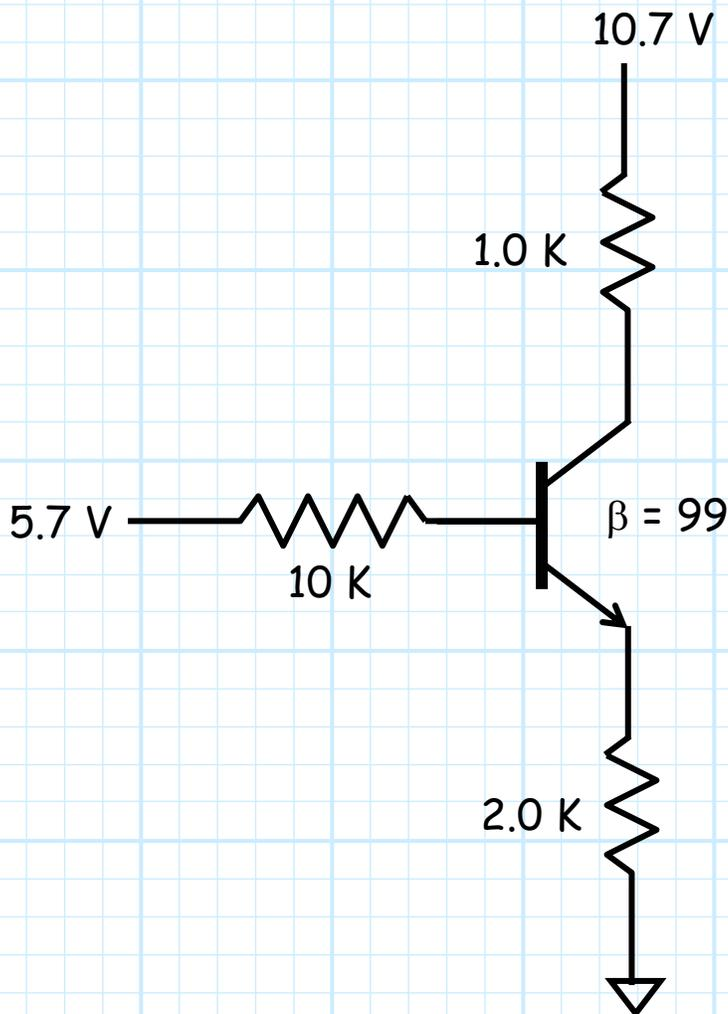
**Q:** What is  $I_B$ ,  $I_C$ ,  $I_E$  and also  $V_{CE}$ ,  $V_{CB}$ ,  $V_{BE}$ ??
