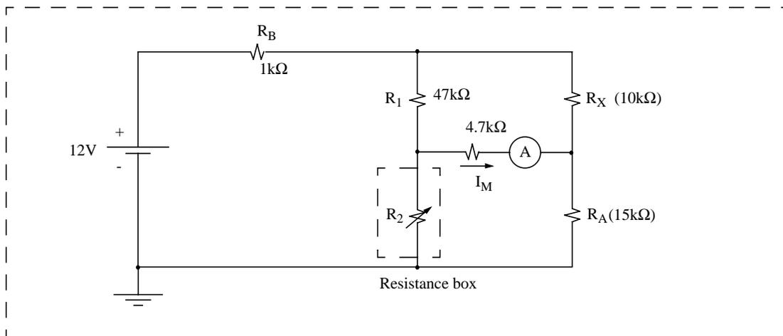
Figure I-A.1: Wheatstone bridge setup
