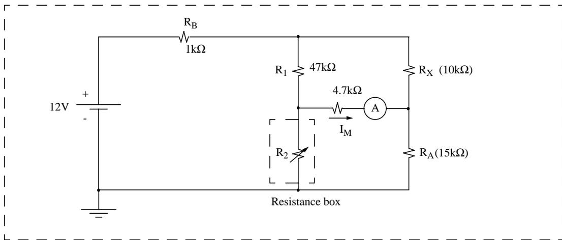
Figure I-A.1: Wheatstone bridge setup
