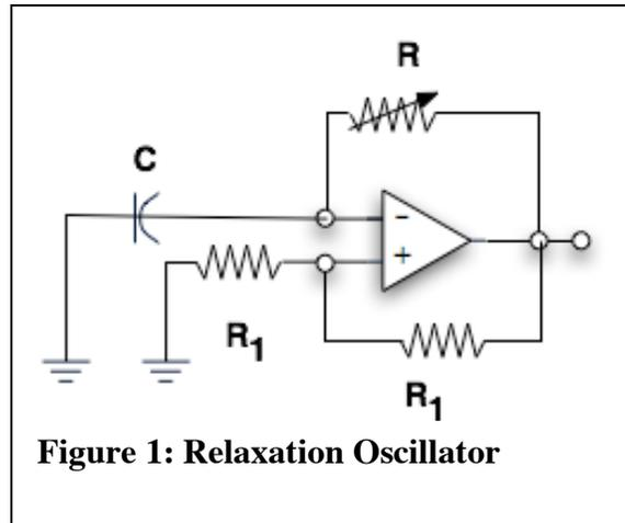
Build the relaxation oscillator shown in Figure 1 above. The output should be a square wave with a frequency about  $1/(2RC)$ . Resistor  $R_1$  can be any value between 1K and 1 M. Resistor  $R$  is one side of a potentiometer. Examine the voltages at (+) and (-) inputs and at the output and follow the action of the switching. It is useful to display  $v_+$  and  $v_-$  simultaneously on the same scale to illustrate that the switching occurs at the crossover of  $v_+$  and  $v_-$ .
