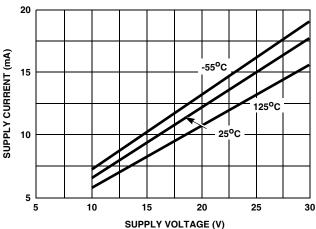
FIGURE 11. SUPPLY CURRENT vs SUPPLY VOLTAGE
