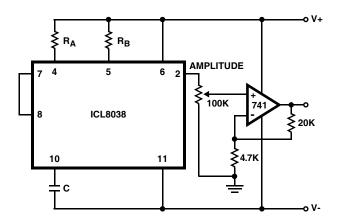
FIGURE 6. SINE WAVE OUTPUT BUFFER AMPLIFIERS
