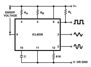
FIGURE 5B. CONNECTIONS FOR FREQUENCY SWEEP FIGURE 5.
