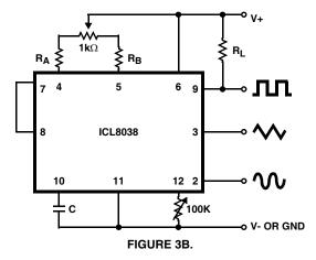
FIGURE 3. POSSIBLE CONNECTIONS FOR THE EXTERNAL TIMING RESISTORS
