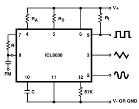
FIGURE 5A. CONNECTIONS FOR FREQUENCY MODULATION
