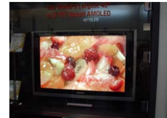
40" AMOLED using a-Si technology Courtesy of Samsung Electronics
