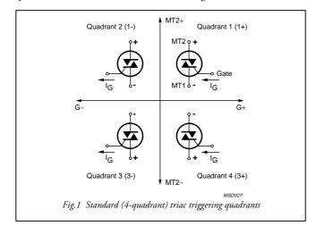
This triggering versatility arises from the fact that the gate consists of some elements that conduct temporarily during the turn-on phase. In particular, one of the triggering modes, 3+ (or quadrant 4), relies on the main terminal 1 supplying electrons to trigger a thyristor element in the gate-MT1 boundary. Conduction then spreads to the main thyristor element from this boundary.
