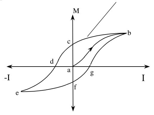
a-b : initial magnetization, saturation at b
