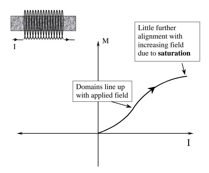
As the current in the coil is increased, initially large numbers of domains align with the externally applied field: there is a torque on the dipoles of unaligned domains.
