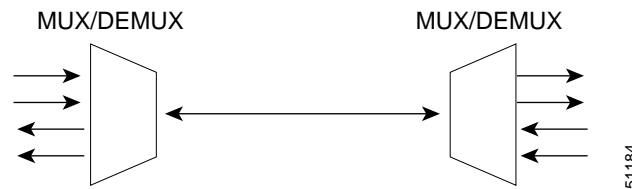
Figure 2-19 Multiplexing and Demultiplexing in a Bidirectional System
