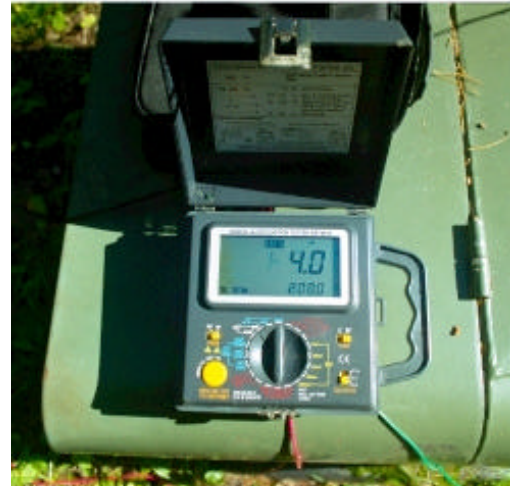
TPI MFT5010 Instrument Showing the 50 foot reading of 4.0 Ohms.
