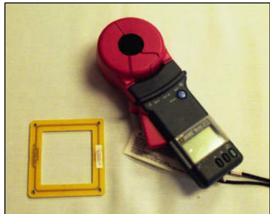
Clamp-On Type Ground Tester Shown with calibration loop
