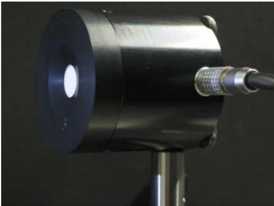
Figure 4. The standard photometer LMT P11 SOT.
