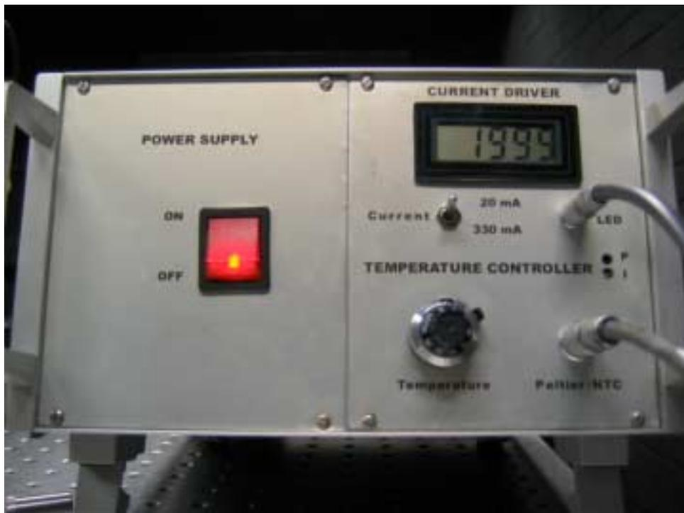
Figure 3. The LED control unit.
