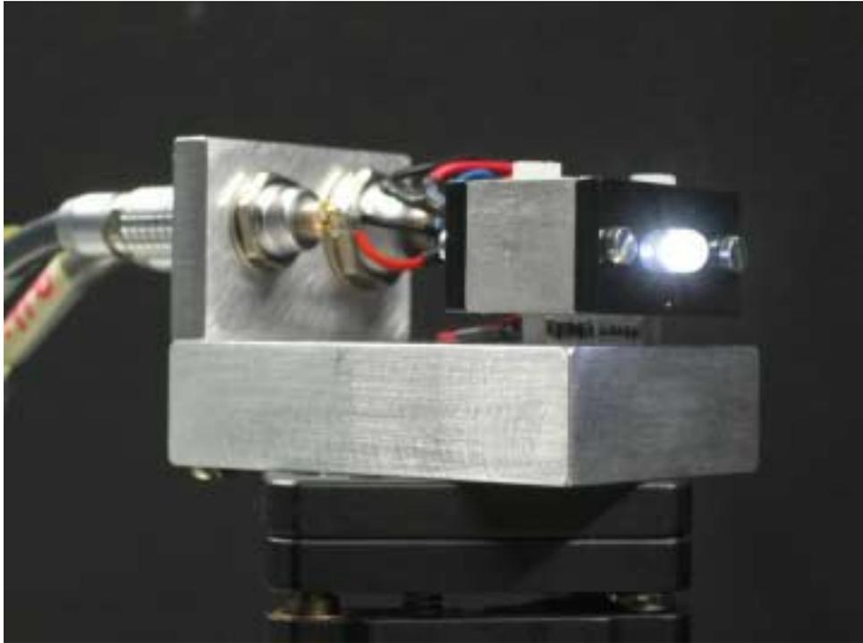
Figure 1. A white standard LED. The temperature of the LED is stabilized with a Peltier element.
