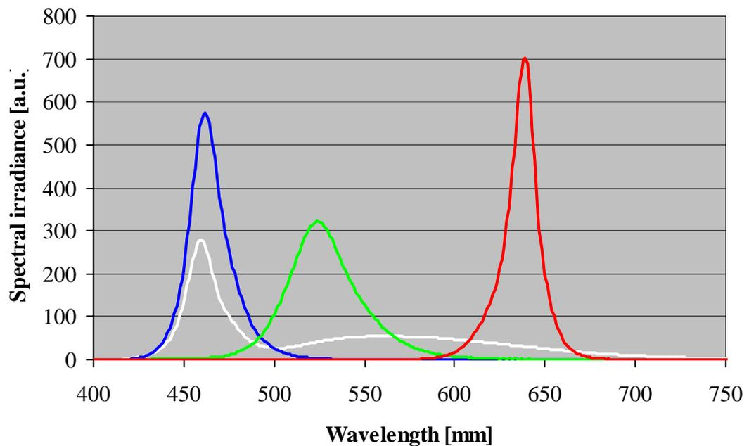
Figure 2. The relative spectral power distributions of the standard LEDs. The peak intensities are not to scale.
