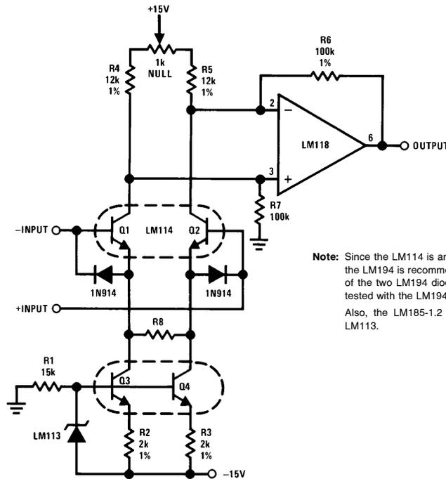
**Note:** Since the LM114 is an obsolete part, substitution of the LM194 is recommended, along with the removal of the two LM194 diodes. This circuit has not been tested with the LM194 included.
