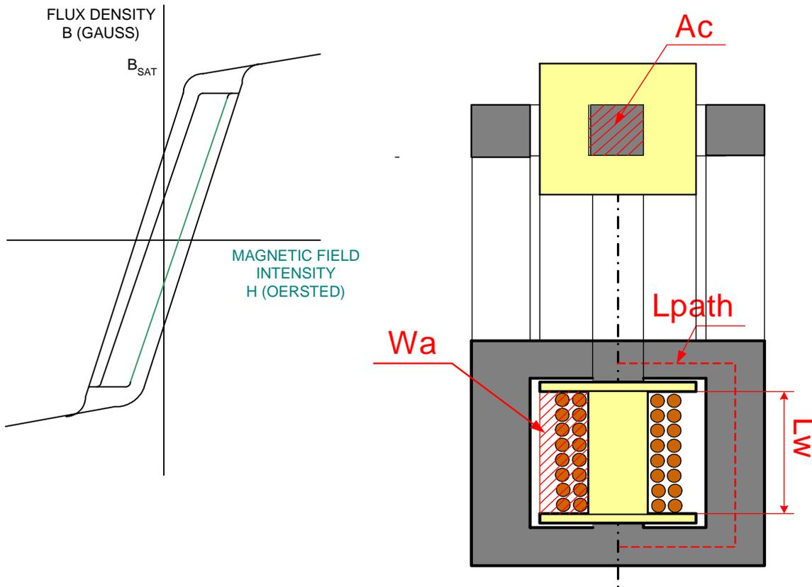
The power handling capacity of the transformer core can be determined by its  $W_a A_c$  product area, where  $W_a$  is the available core window area, and  $A_c$  is the effective core cross-sectional area. The  $W_a A_c$  power output relationship is obtained with the Faraday's law:
