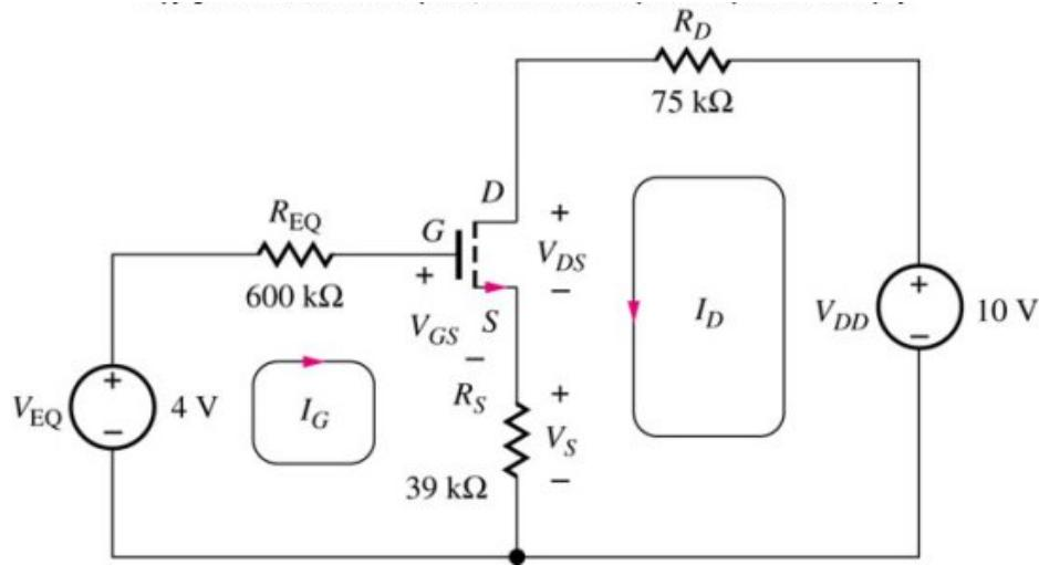
Since  $I_G=0$ ,  $V_{EQ}=V_{GS}+I_D R_S$
