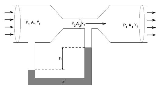
The centers of all the tubes have a common elevation; therefore the gravity-terms drop out of Bernoulli's equation. This leaves
