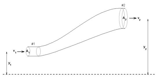
The total mechanical energy of the volume element at position #1,  $E_1$ , is
