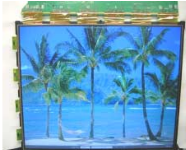
Figure 1: A 17" SXGA PC monitor using the Solomon Systech SSD1205 and SSD1237 gate and source driver ICs
